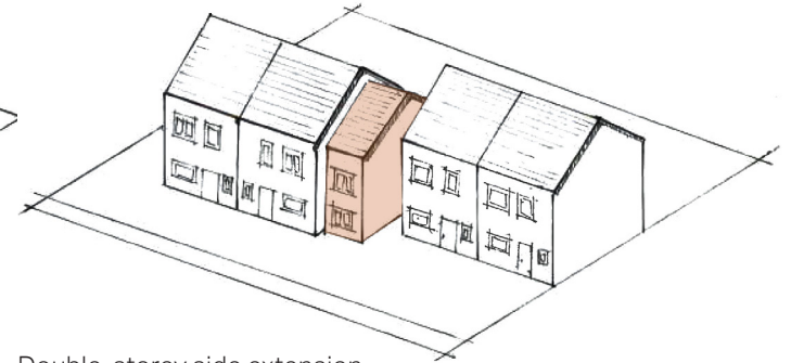
Double-storey side extension
